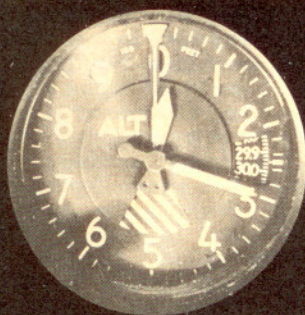
Figure 1. A modern three-pointer-type sensitive altimeter, showing a barometric-pressure setting of 29.95 in. Hg. and an indicated altitude of 300 feet ms1. The barber-pole-striped sector of the dial will be masked when the airplane is at approximately 16,000 feet.
