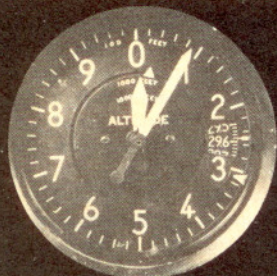
Figure 2. A sensitive altimeter with triangular airport-altitude reference marks. In this illustration, an airport altitude of 310 feet has been set into the instrument. When the airplane is on the ground, the pointers will indicate zero.
